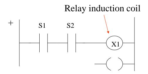
In the contact (ladder) diagram only the coil of the relay is represented
