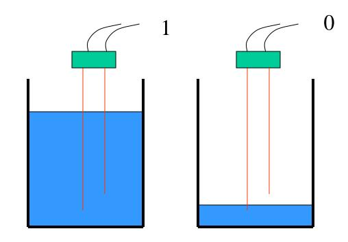
Closed Open circuit circuit
