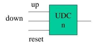
The output is activated when the input changes from false to true n times. The counter is reset to zero when the reset input is activated.
