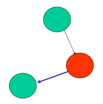
Transitions between states are formulated as logic functions of the system variables or time. A transition can be activated when the system is in the previous state and the logic condition is true. Each state have a set of associated actions.
