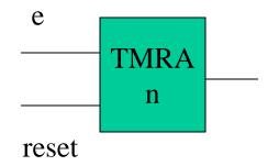
**Ton, Tof** Timer on/off Delay. The output is activated n time units after the input is activated. The timer is reset if the input does not keep active for n seconds
