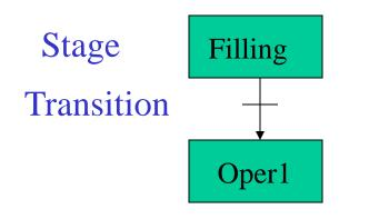
When the logic condition associated to a transition becomes true (and the process is in the corresponding stage), the current stage is deactivated and the following one is activated, besides executing all its associated actions. The logic condition can be formulated in any of the IEC 61131 languages
