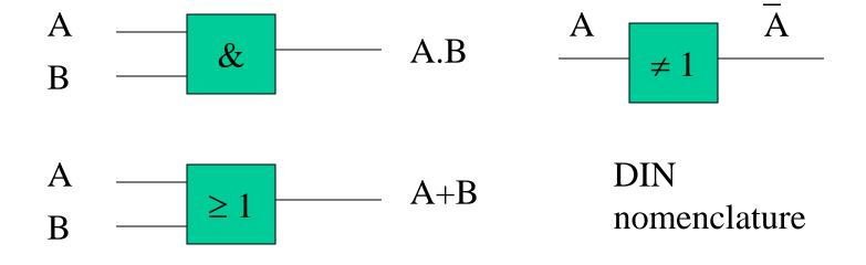
Logic expressions can be assimilated to electrical circuits where true/false can be represented by the presence or not of an electrical signal and the conclusion is expressed in terms of the value of the output signal
