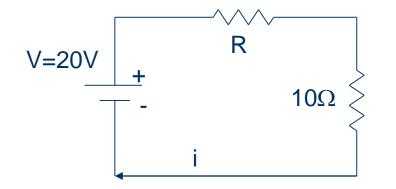
Find the value of R so that the power dissipated in this resistor is maximized
