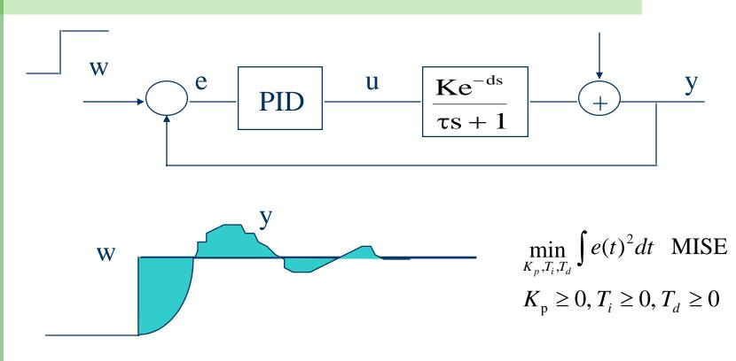
error = w - y (linear function of  $K_p$ ,  $T_i$ ,  $T_d$ )
